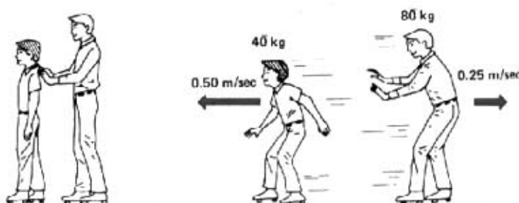
Figure 9.2.1.2 Conservation of momentum. On a frictionless surface, the momentum of the boy toward the left is equal to the momentum of the man toward the right.
